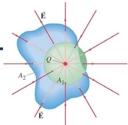
A single point charge surrounded by a spherical surface,  $A_1$ , and an irregular surface,  $A_2$ .
